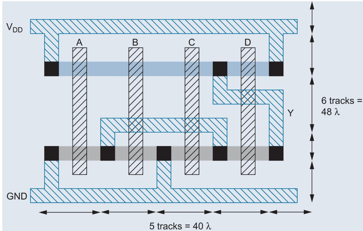
**FIG 1.47** CMOS compound gate for function  $Y = (A + B + C) \cdot \overline{D}$
