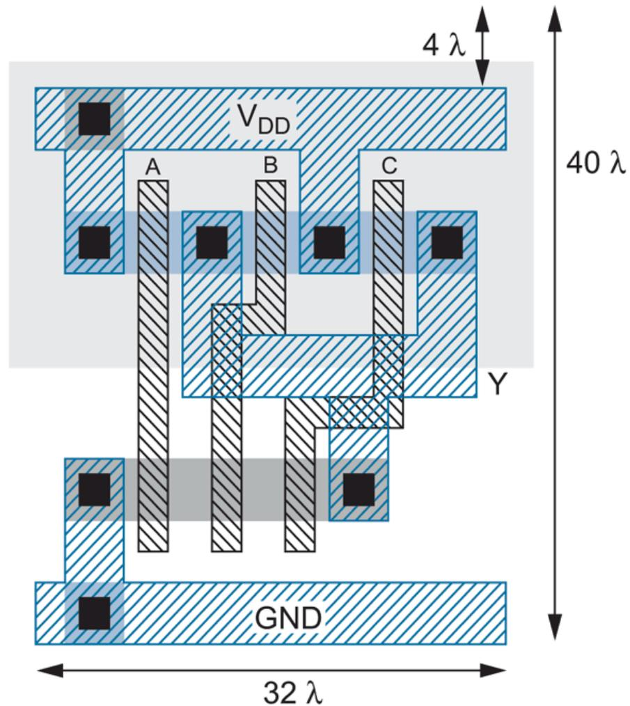
**FIG 1.42** 3-input NAND standard cell gate layouts
