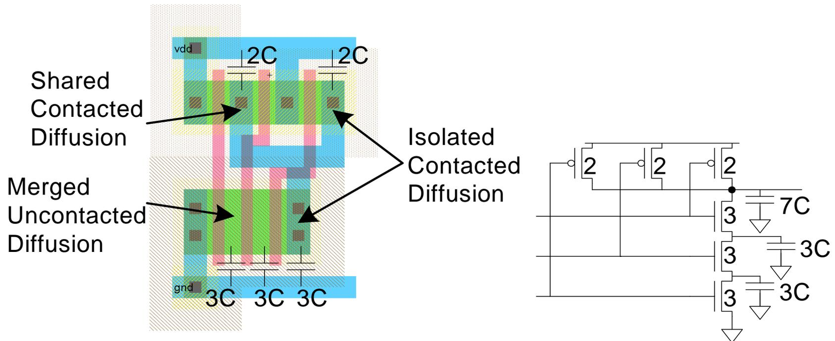
*RC Delay Models: Layout Comparison*
