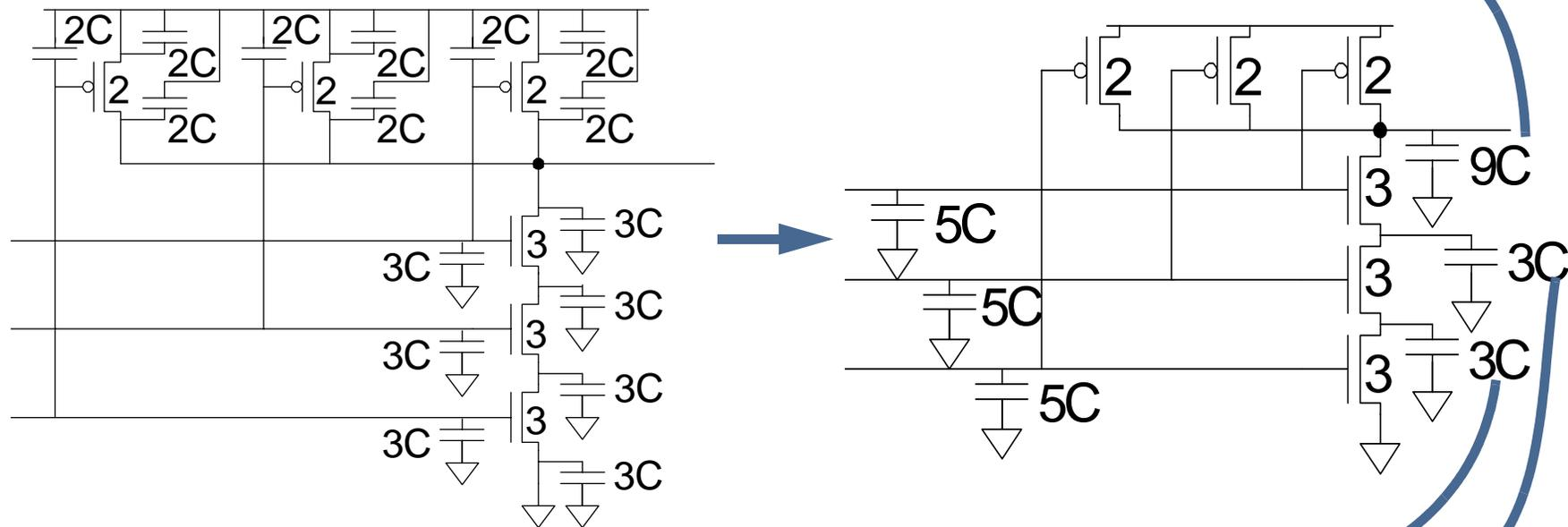
Conservative estimate would assume that this two diffusions are uncontacted and therefore have lower capacitance (the difference is usually ignored for hand calculations)
