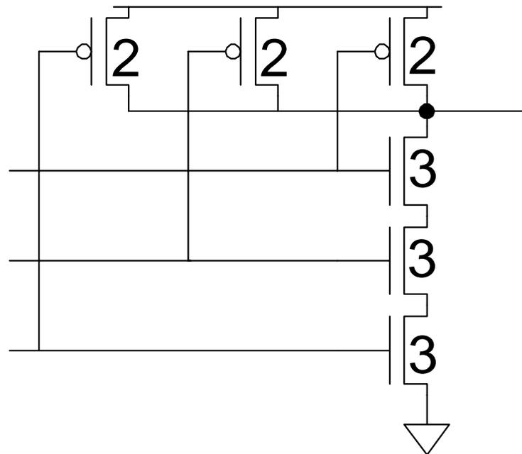
3 NMOS in series =  $3R$ , therefore each has to be three times the minimum width.
