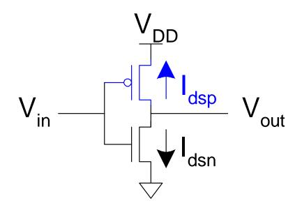
$$V_{gsp} = V_{in} - V_{DD}$$
