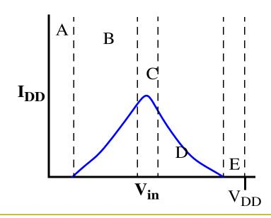
Supply current I<sub>DD</sub> vs. V<sub>in</sub>.
