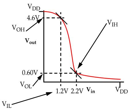
$$NM_H = V_{OH} - V_{IH} = 4.6V - 2.2V = 2.4V$$
