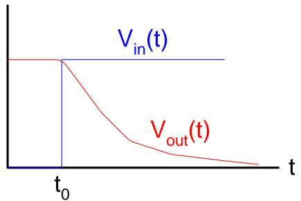
$$I_{dsn}(t) = \begin{cases} \frac{\beta}{2} (V_{DD} - V)^2 \\ \beta (V_{DD} - V_t - V_{out}(t)/2) V_{out}(t) \end{cases}$$
