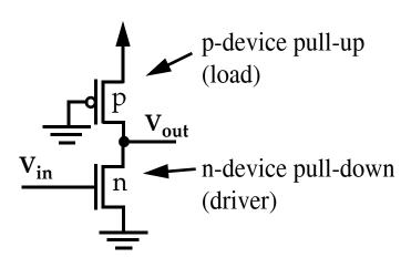
When driver is on, steady-state current flows - not a good choice for low-power circuits.
