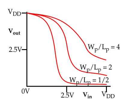
Therefore, the shape of the transfer characteristic and the  $V_{OL}$  of the inverter is affected by
