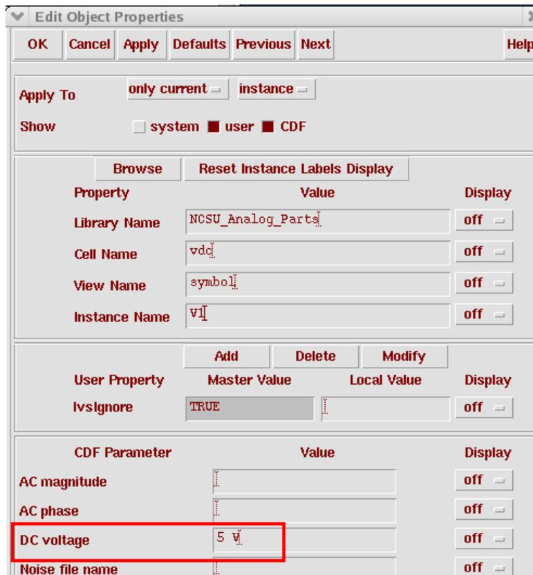
Figure 5: Property of vdc used for the simulation
