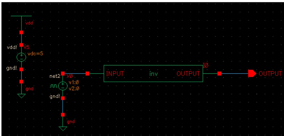
Figure 4: Schematic of inv\_sim
