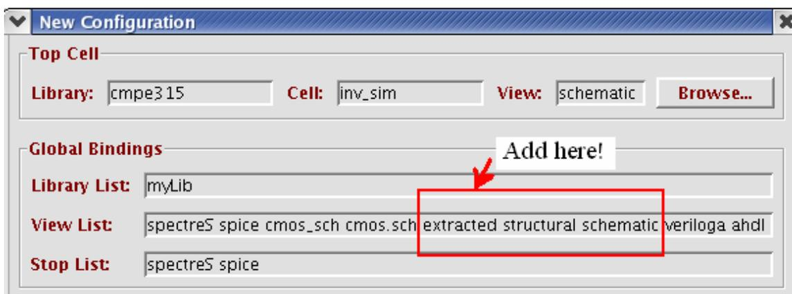
Figure 10: Add "extracted structural schematic" to View List
