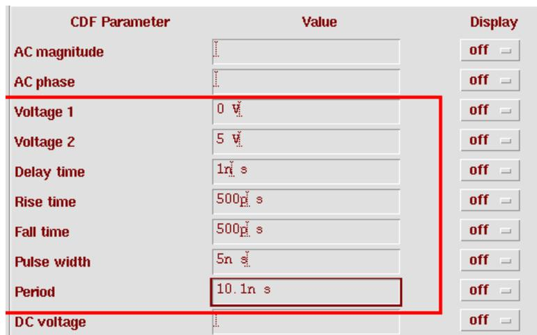
Figure 6: Property of vpulse used for the simulation
