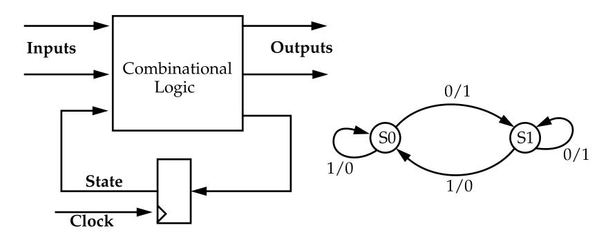
Combinational part implemented in one process, sensitive to events on the input signals or state variables.
