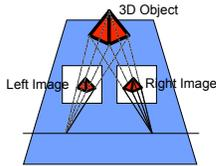
1. Stereo camera calibration → compute camera relative pose
