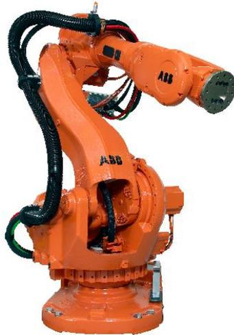
Fig. 1.1 The ABB IRB6600 Robot. Photo courtesy of ABB.
