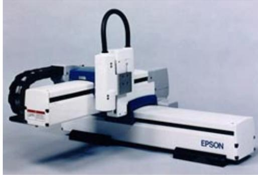
Fig. 1.20 The Epson Cartesian Robot. Photo courtesy of Epson.
