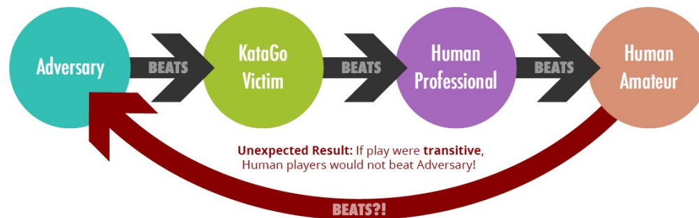
Figure 2.1: A human amateur beats our adversarial policy (Appendix I.1) that beats KataGo. This non-transitivity shows the adversary is not a generally capable policy, and is just exploiting KataGo.
