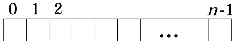
$$\text{bit}[i] = \begin{cases} 0 \Rightarrow \text{block}[i] \text{ free} \\ 1 \Rightarrow \text{block}[i] \text{ occupied} \end{cases}$$
