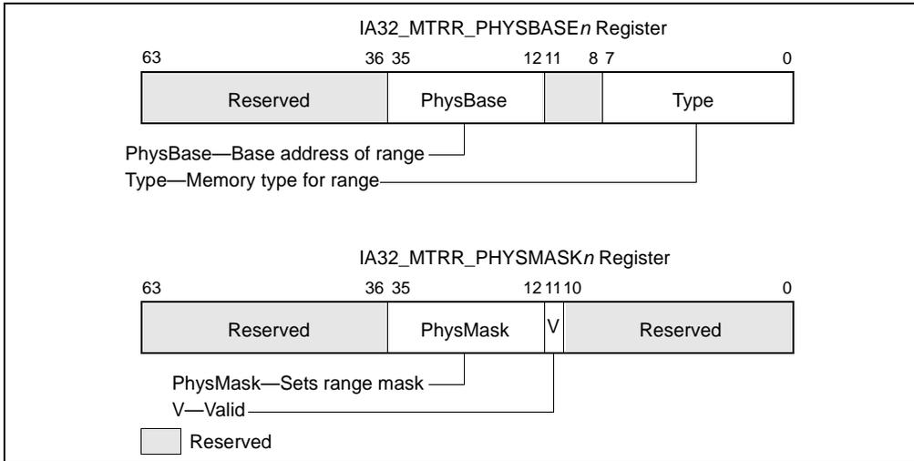
**Figure 9-6. IA32\_MTRR\_PHYSBASE<sub>n</sub> and IA32\_MTRR\_PHYSMASK<sub>n</sub> Variable-Range Register Pair**
