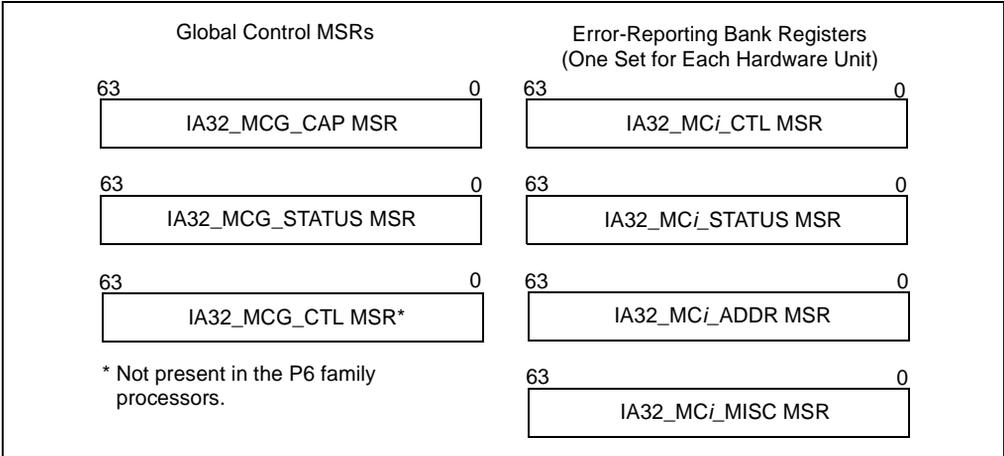
Figure 13-1. Machine-Check MSRs
