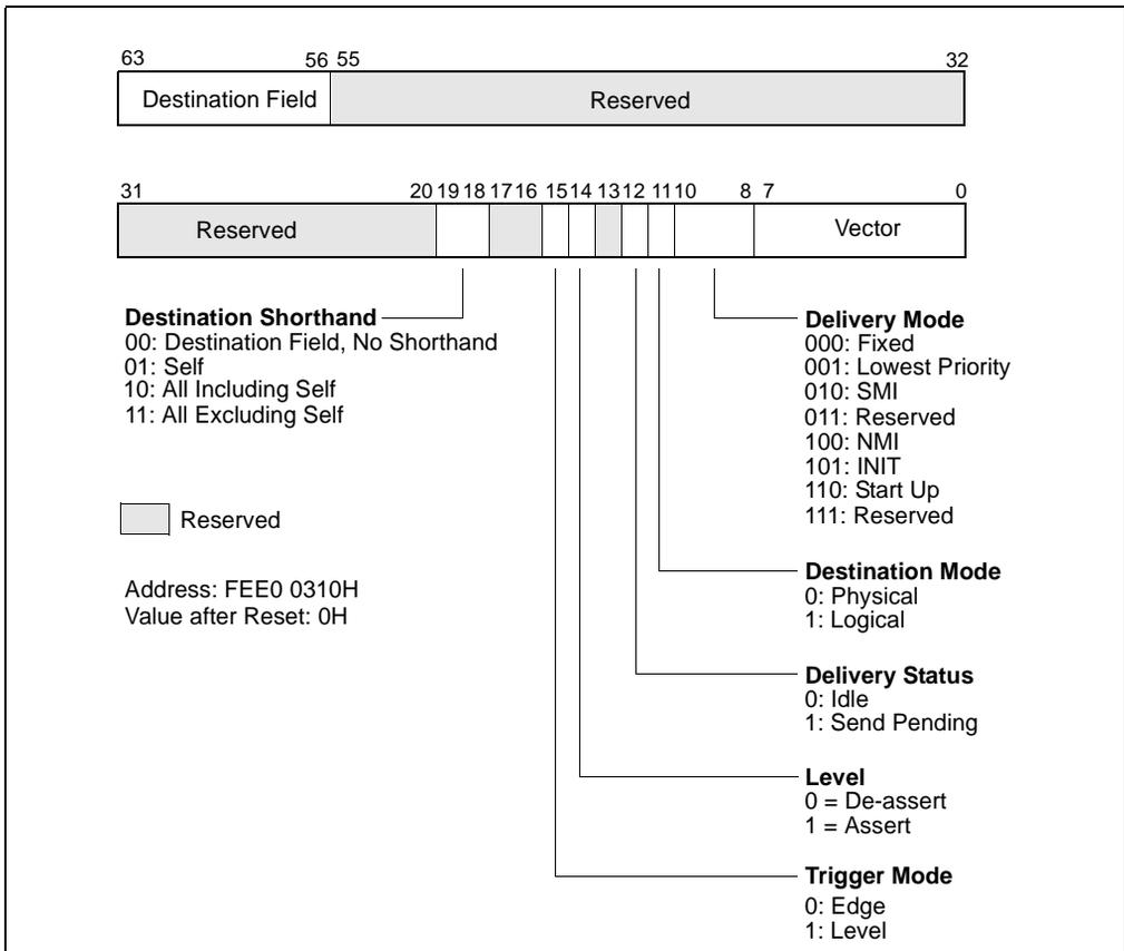
Figure 7-10. Interrupt Command Register (ICR)
