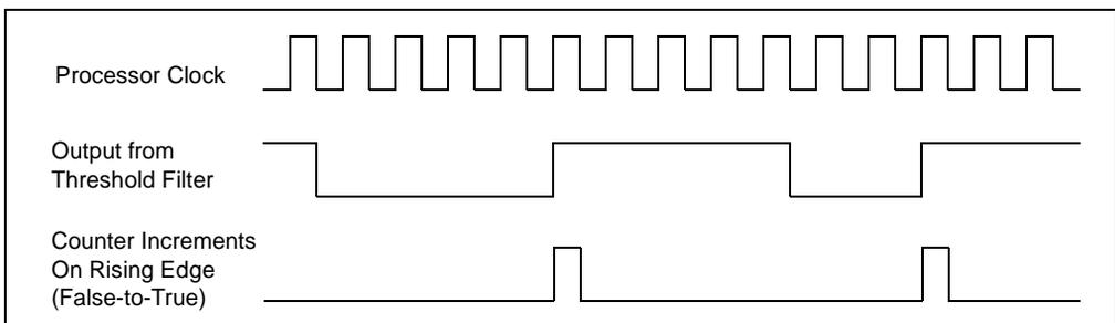
**Figure 14-14. Effects of Edge Filtering**
