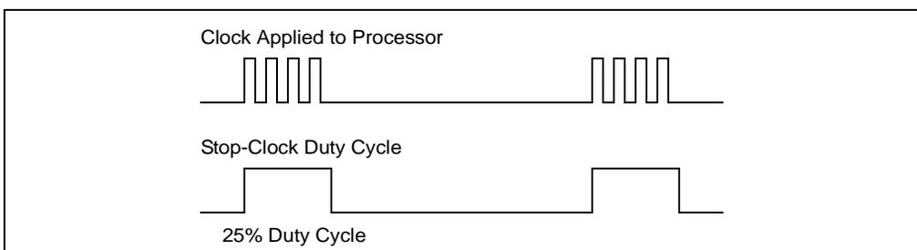
**Figure 12-6. Processor Modulation Through Stop-Clock Mechanism**
