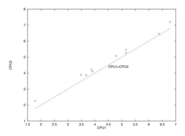
This plots CPU1 versus CPU2 and also plots the line y = x. Notice that the performance of CPU1 is correlated with the performance of CPU2. Notice that all points lie above the line, suggesting that CPU2 is always bigger than CPU1.
