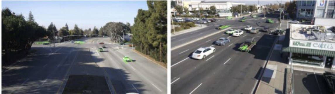
Real-time tracking of vehicles with optical flow. Source
