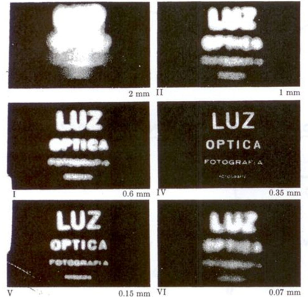
Fig. 5.96 The pinhole camera. Note the variation in image clarity as the hole diameter decreases. [Photos courtesy Dr. N. Joel, UNESCO.]
