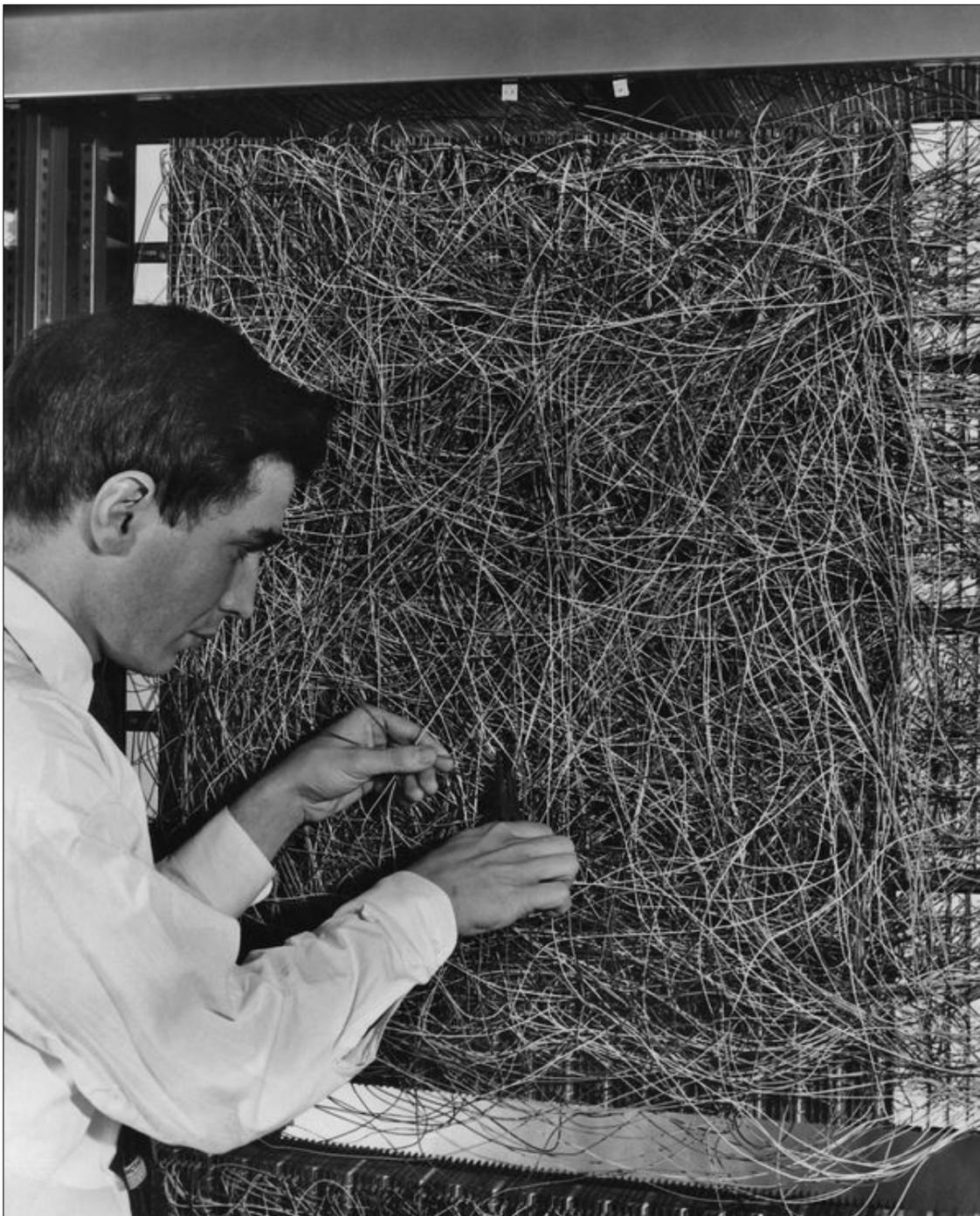
A man adjusting the random wiring network between the light sensors and association unit of scientist Frank Rosenblatt's [Perceptron](#), or MARK 1 computer, at the Cornell Aeronautical Laboratory, Buffalo, New York, circa 1960. The machine is designed to use a type of artificial neural network, known as a perceptron.
