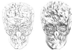
Figure 9: Registration of C towards B. Left, we see the deformed set C with B. The matched points are linked. Notice how the two sets are well superimposed. Right, C is in its original position. It allows to estimate the extent of the deformation between the two sets.
