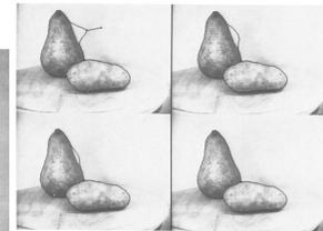
Fig. 4. Two edge snakes on a pear and points. Upper-left: The user has pulled one of the snakes away from the edge of the pear. Other: After the user lets go, the snake snaps back to the edge of the pear.
